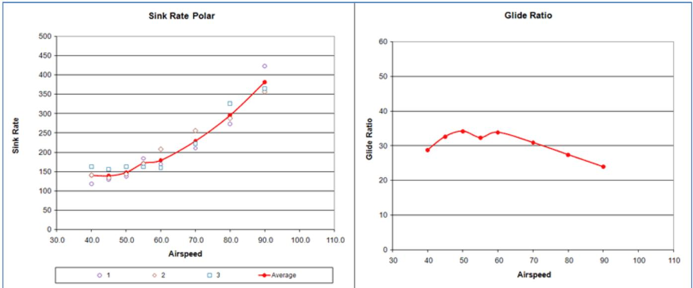
Figure 5 - Sink Rate and Glide Ratio Plots
